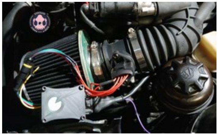
An example of an installed kit using internal IAT.
